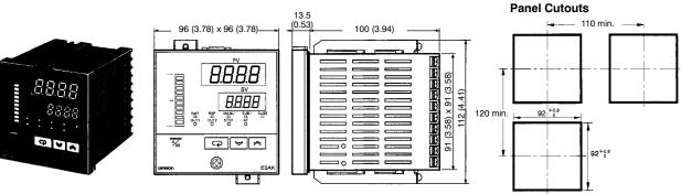
Note: 1. Recommended panel thickness is 1 to 8 mm.
